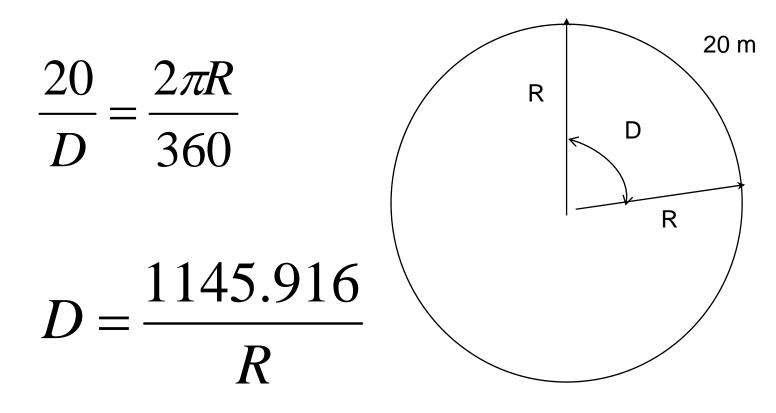
In practice the design engineer usually selects the degree of curvature on the basis of such factors as the design speed and allowable superelevation. Then the radius is calculated.
