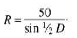
For a 10 curve (chord definition), D = 1; therefore R = 5,729.65 feet, or meters, depending upon the system of units you are using.
